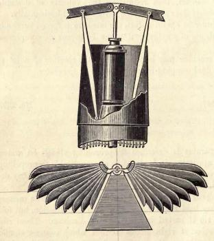
The boiler is constructed with a number of small tubes to give a large heating surface with small amount of weight, as well as requiring a very small amount of water; and the heat is obtained by burning vaporized hydrocarbon combined with a hot-air blast. The exhaust steam is condensed in a hollow tail, thus saving weight in the quantity of water required. This tail also serves the purpose of a supporting surface (i. e. aëroplane).
